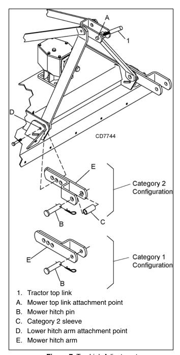
Figure 7. Top Link Adjustment
